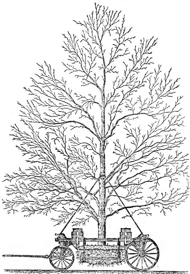
Machine used in Brooklyn and at Washington for transplanting large trees.
