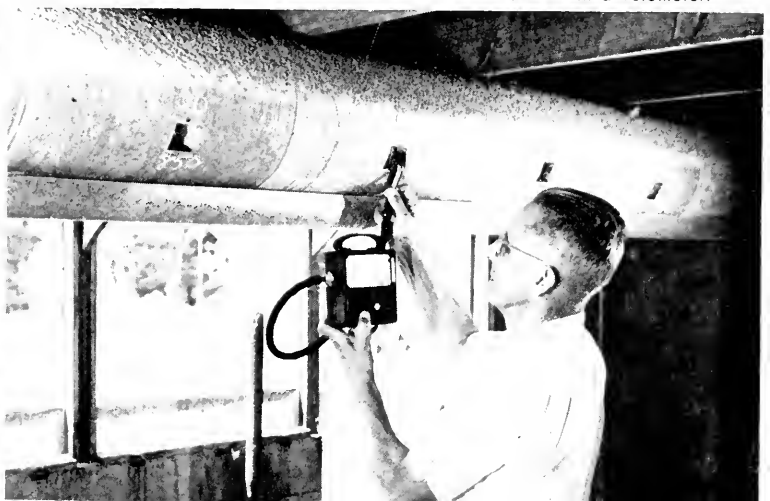
VENTILATION STUDIES. The University has recently developed a new ventilation system that provides a uniform and controlled flow of air in animal pens. Here the rate of air movement is checked with a velometer.
