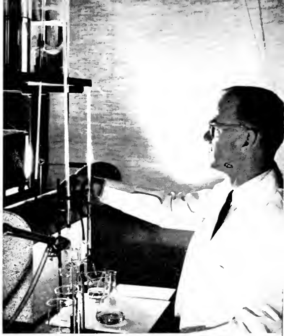
Determining volatile acids and bases as a measure of quality in silage.
