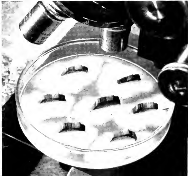
5. Diagnosing and Recording Results: After a few days fungus in the wood may be identified by its growth in the culture dishes.
