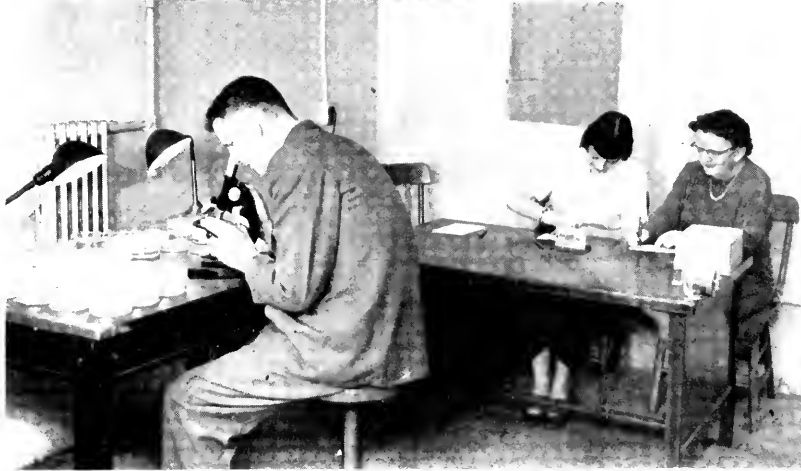
5. Diagnosing and Recording Results: After a few days fungus in the wood may be identified by its growth in the culture dishes.
