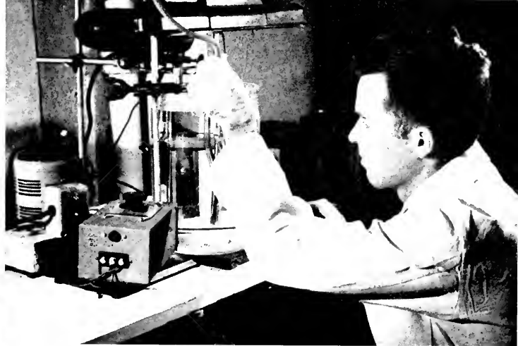
Bacteria are responsible for certain vital chemical changes, but industry must be alert to control the physical changes. Here the viscometer measures the degree of physical change that a product undergoes.
