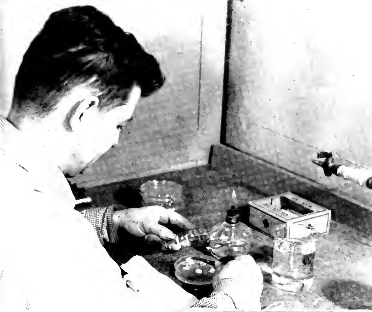
4. Testing: Chips of wood are placed on special fungus food in culture dishes.
