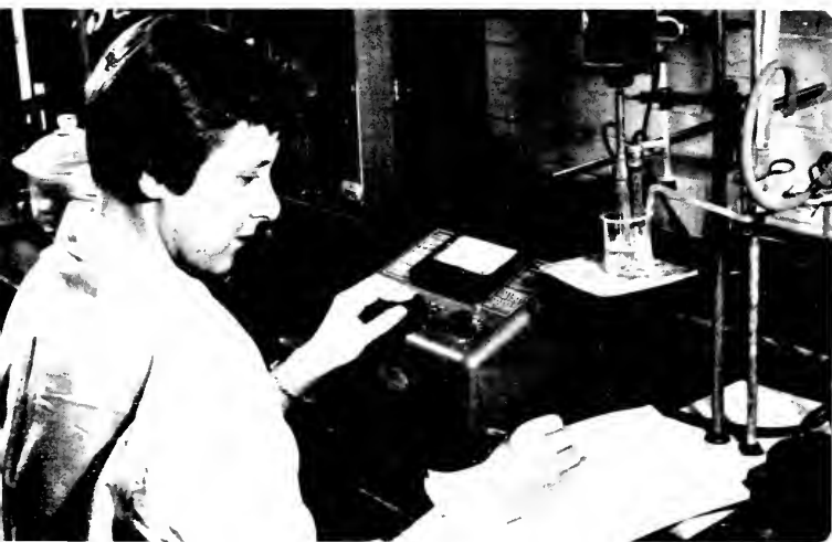
Vinegar producers are always looking for better methods to improve their product. Here the pH meter measures the amount of acid in a product during fermentation.
