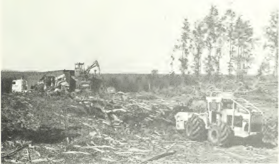
Figure 9.—Landing site showing chain flailing of trees prior to whole-tree chipping—Case III.
