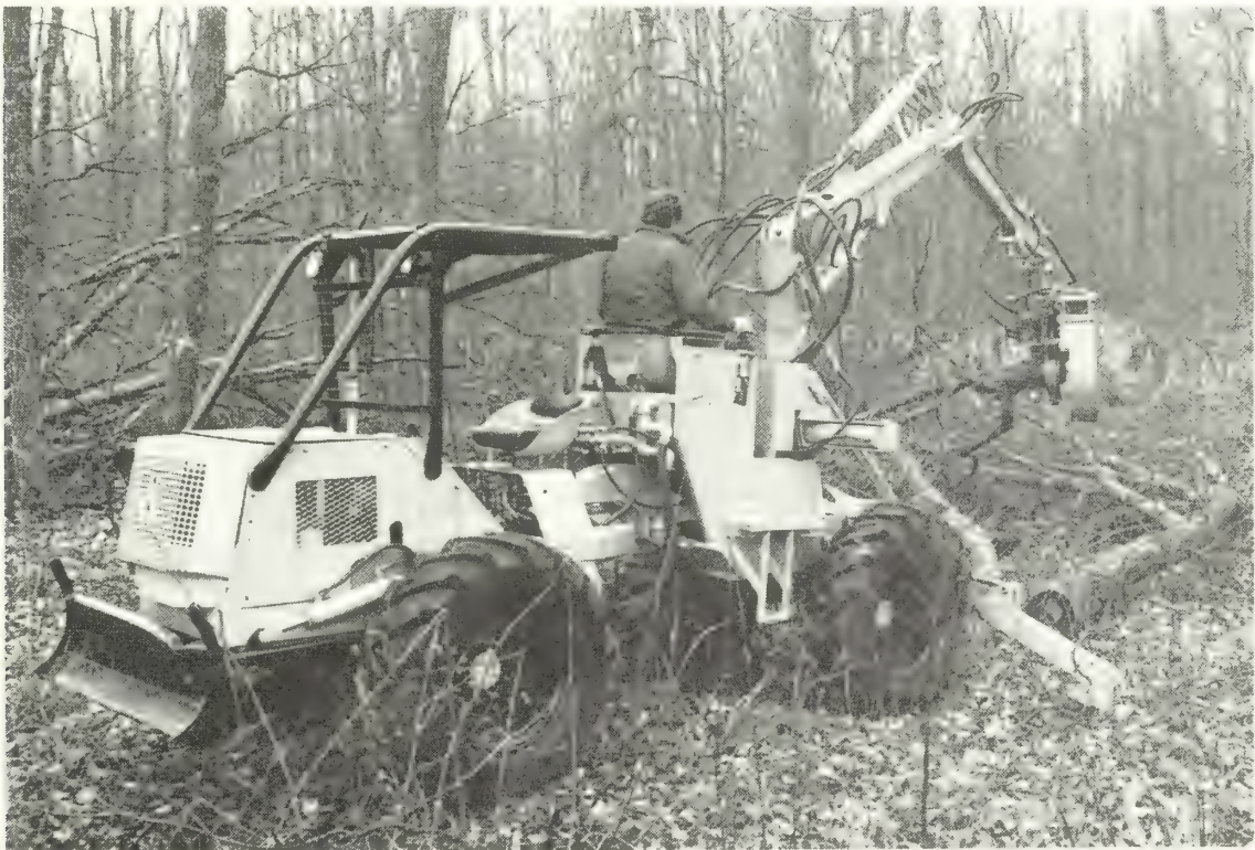
Figure 12.—Experimental topwood processor used for compacting hardwood saw log tops and limbs prior to skidding—Case V.
