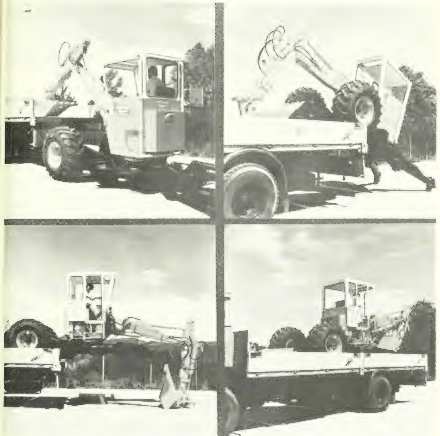
Figure 1.—The Menzi Muck being loaded onto the bed of a transport vehicle (photos courtesy of Climbing Hoe of America, Ltd.).
