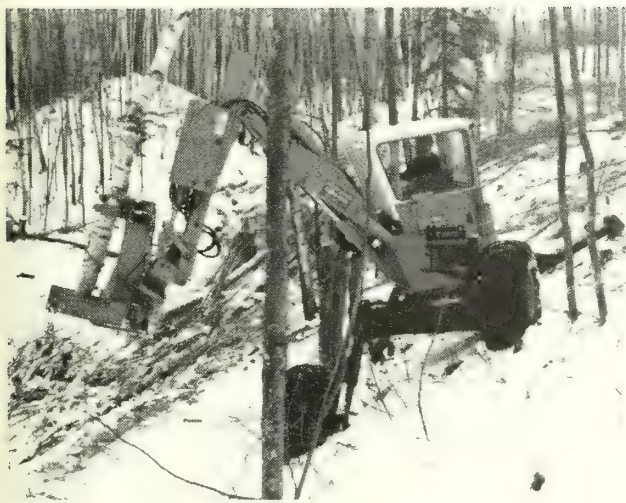
Figure 3.—The Menzi Muck as a small-tree feller/buncher operating parallel to the slope on the pole-sized steep site.
