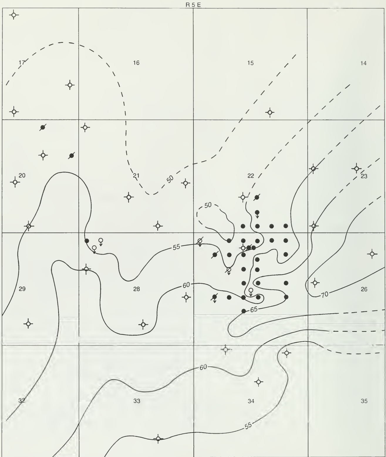
Figure 7 Isopach map of the Aux Vases Formation reveals regional thinning north and northwest of the field. Note the thickness of the Aux Vases along the southeastern portion of the field area and the relatively abrupt thinning within the field. Contour interval is 5 feet.
