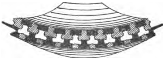
PLAN SHOWING LAYER OF CONCRETE BLOCKS
