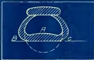
Fig. 7- Showing Change in Form of Meridian Section of Insufficiently Inflated Tire.
