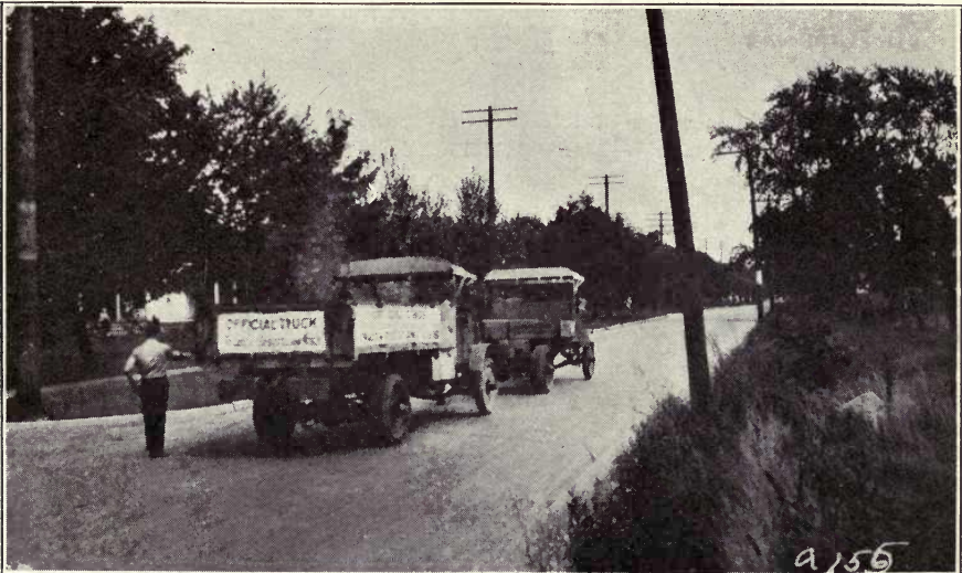
FIG. 1. DAVIDSON DYNAMOMETER AND METHOD OF TOWING
