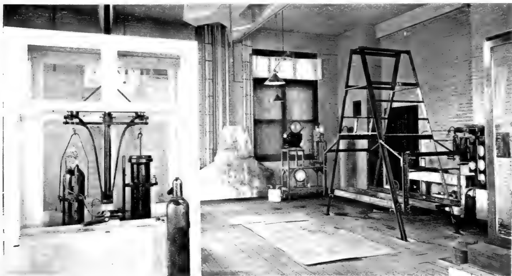
General view of laboratory taken near the temperature recorder. The bed calorimeter is at the right, the absorber table in the immediate foreground, back of it the chair calorimeter and observer's table, and at the left the balance for weighing absorbers. Near the ceiling are shown the ducts for the cold air used for temperature control.
