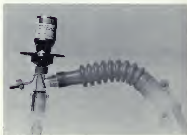
Fig. 14. Instrumentation Industries RTC-21 MDI adapter.
