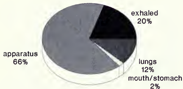
Fig. 5-A. Deposition from small volume nebulizer. (Adapted, with permission, from data in Reference 34.)
