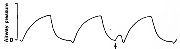
Fig. 2. Estimation of auto-PEEP by the occlusion technique. The expiratory port of the ventilator circuit is occluded at end-expiration (arrow), causing equilibration of pressure in the lungs and ventilation circuit. The pressure registered on the ventilator manometer provides an estimate of the level of auto-PEEP. (Reproduced, with permission, from Reference 12.)
