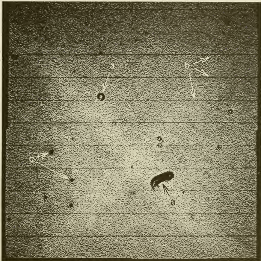
Figure 8. Example of WFPC 2 flat. This is a 400 \times 400 pixel section from the center of detector WF2 for filter F555W. The gray scale ranges from 0.95 (black) to 1.05 (white). Data are from ground-based camera tests. Some notable features are: (a) dust particles on windows, (b) 34 row manufacturing error, and (c) dust particles on the CCD itself.
