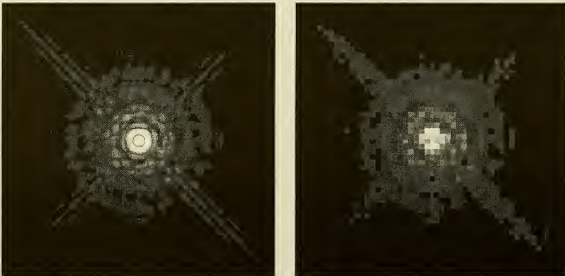
Figure 4. The Tiny Tim PSF ( y filter, F547M) used for generating the image in Fig. 2. To the left (a) the PSF is shown with four times oversampling, to the right (b) with normal sampling. The intensity scale is logarithmic, in order to also show the outer parts of the PSF.
