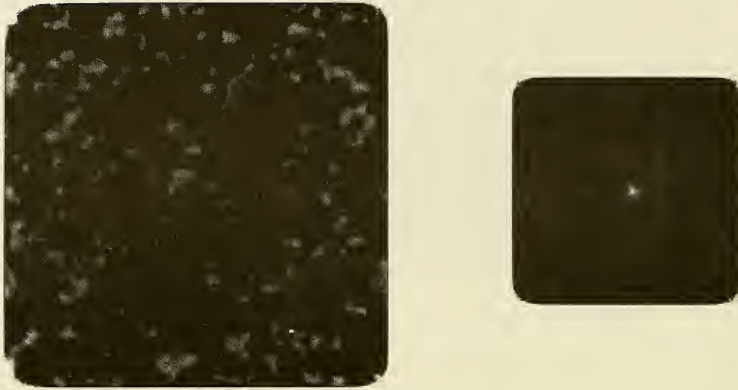
Figure 4. Random test signal and measured point spread function.
