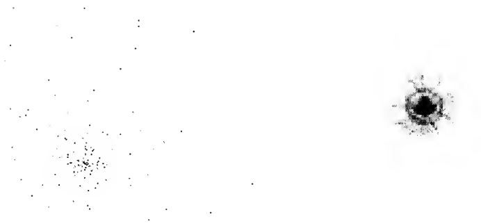
Figure 2. Restored object (left) and restored PSF (right). Note that the PSF is displayed with a factor of 2 magnification.
