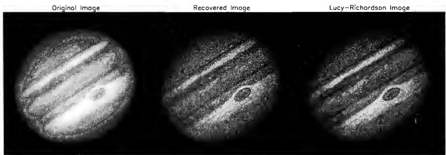
Figure 4. Sample recovery of an HST image of Jupiter compared with a Richardson-Lucy recovery.
