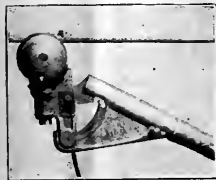
Running Position of the Holmes and Allen Automatic Non-Fouling Swivelling Trolley-Head for Electric Cars.
