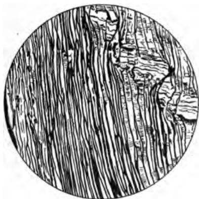
FIG. 34.—Fracture cleavage in slate emphasized by ferruginous staining. There are 360 cleavage planes to the inch. After Dale.
