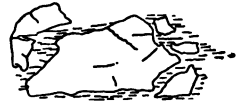
FIG. 26.—The secondary development of parallel sericite by crystallization in cracks formed by fracture. (H. 1040 Sericite-schist. Tamus.)
