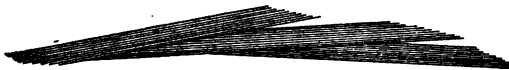
FIG. 2.—Sketch showing the manner in which mica plates feather out, one against the other, in rocks with flow cleavage.
