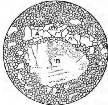
FIG. 10.—Sketch showing granulation of quartz (A) where feldspar (B) is comparatively unaffected by deformation.
