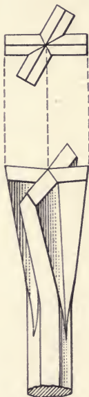
Fig. 26. X Bit Drill Steel
