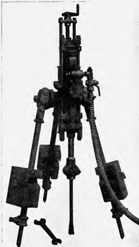
Fig. 17. Rock Drill on Tripod.
