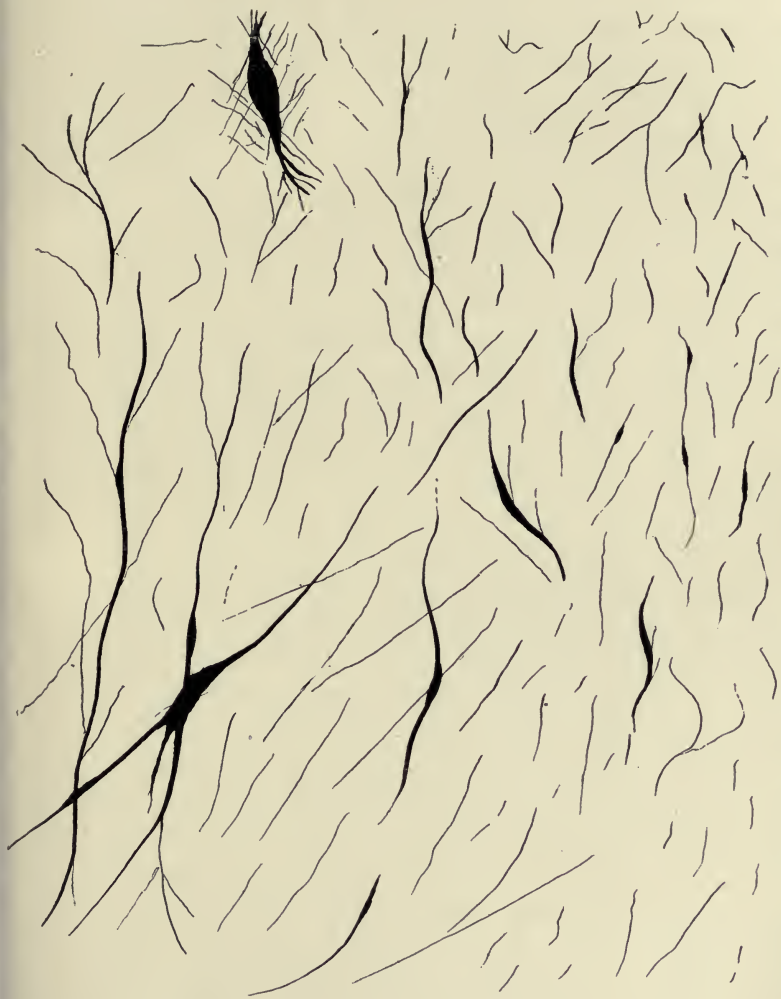
Possible appearance of the surface of a mining camp, with the Lodes Slivers, and Spurs. The possible Commercial Mines represented by the darker lines. The intersection points are often the richest.
