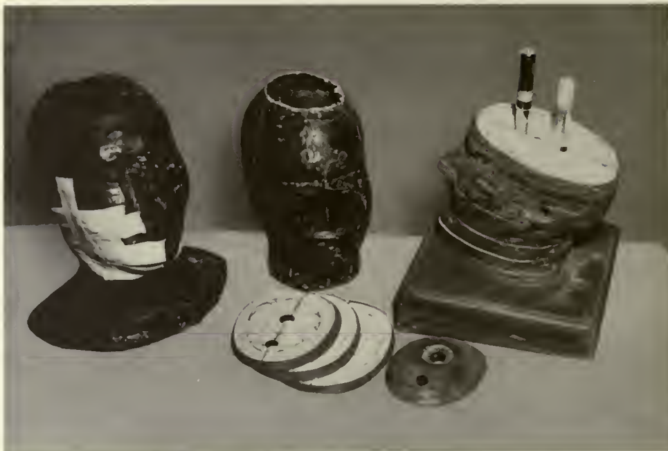
Fig. 9—Phantoms of heads were made with thermosetting material (left) and bonded pressed wood (right).
