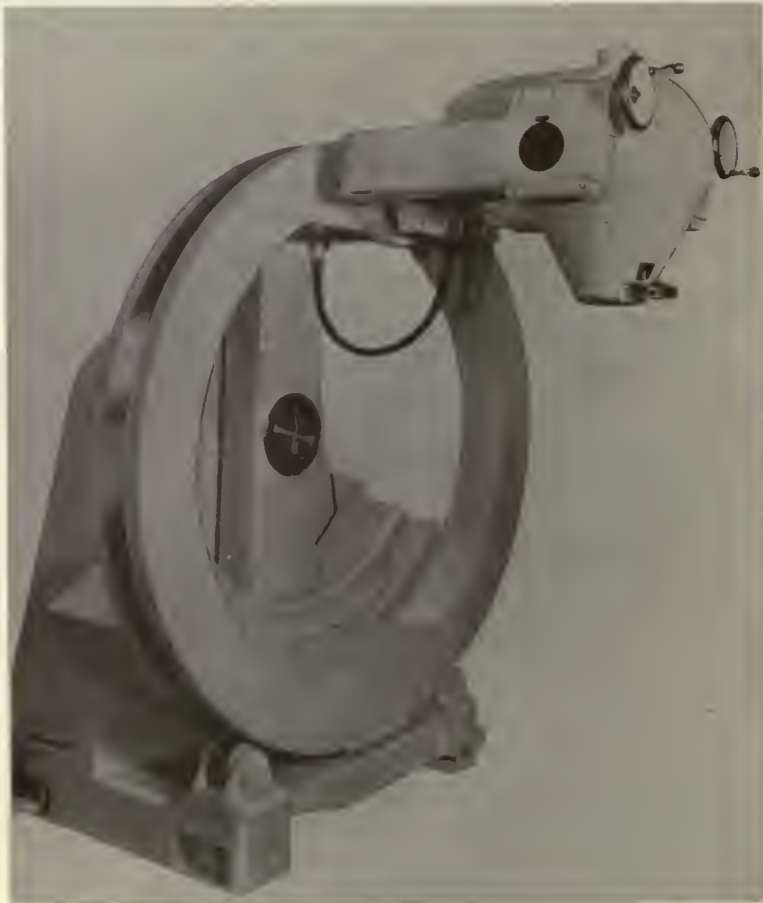
Fig. 7—The Rotaray with rim counterbalance.
