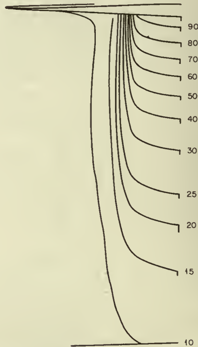
Fig. 9—Source-to-skin distance, 70 cm; source-to-collimator distance, 50 cm; collimator-to-skin distance, 20 cm; field, 10 cm diameter at 70 cm; aperture, 7.4 cm.
