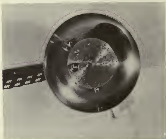
Fig. 2—Vacuum threader as it appears from the top. The circular catch tray prevents spillage of the sources in the course of threading. Note the light illuminating the threading hole.
