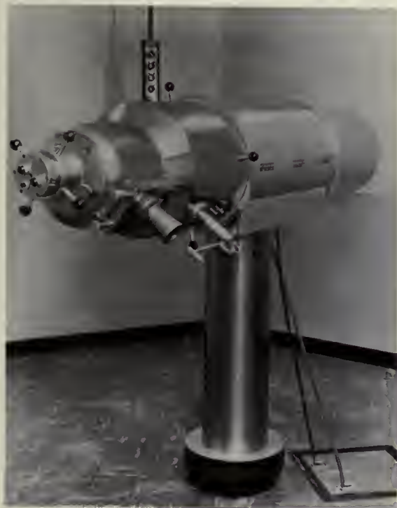
Fig. 2—The City of Hope teletherapy machine mounted on a central pedestal, showing the hydraulic lift mounted in the floor.
