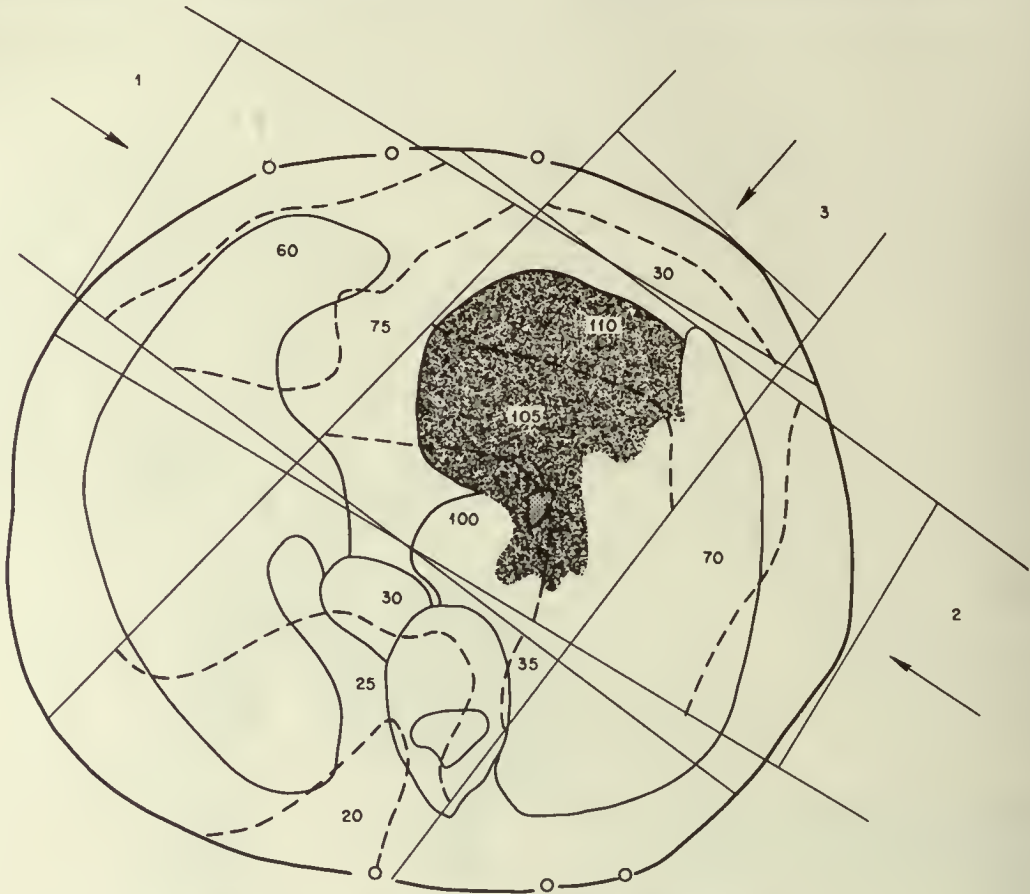
Fig. 14—Isodose curves plotted for heterogeneous tissue (same as Fig. 13.).
