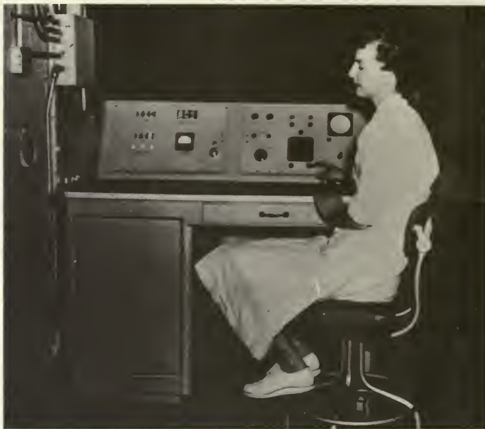
Fig. 10—Control panel. At the left are shown from top to bottom the dose, the time, and the output at the axis of rotation.
