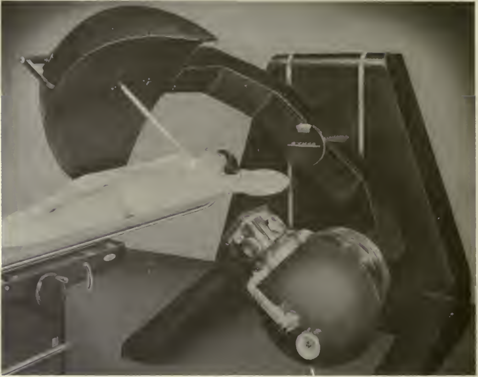
Fig. 4—Picker C-1000 teletherapy unit for a 1000-rhm source.
