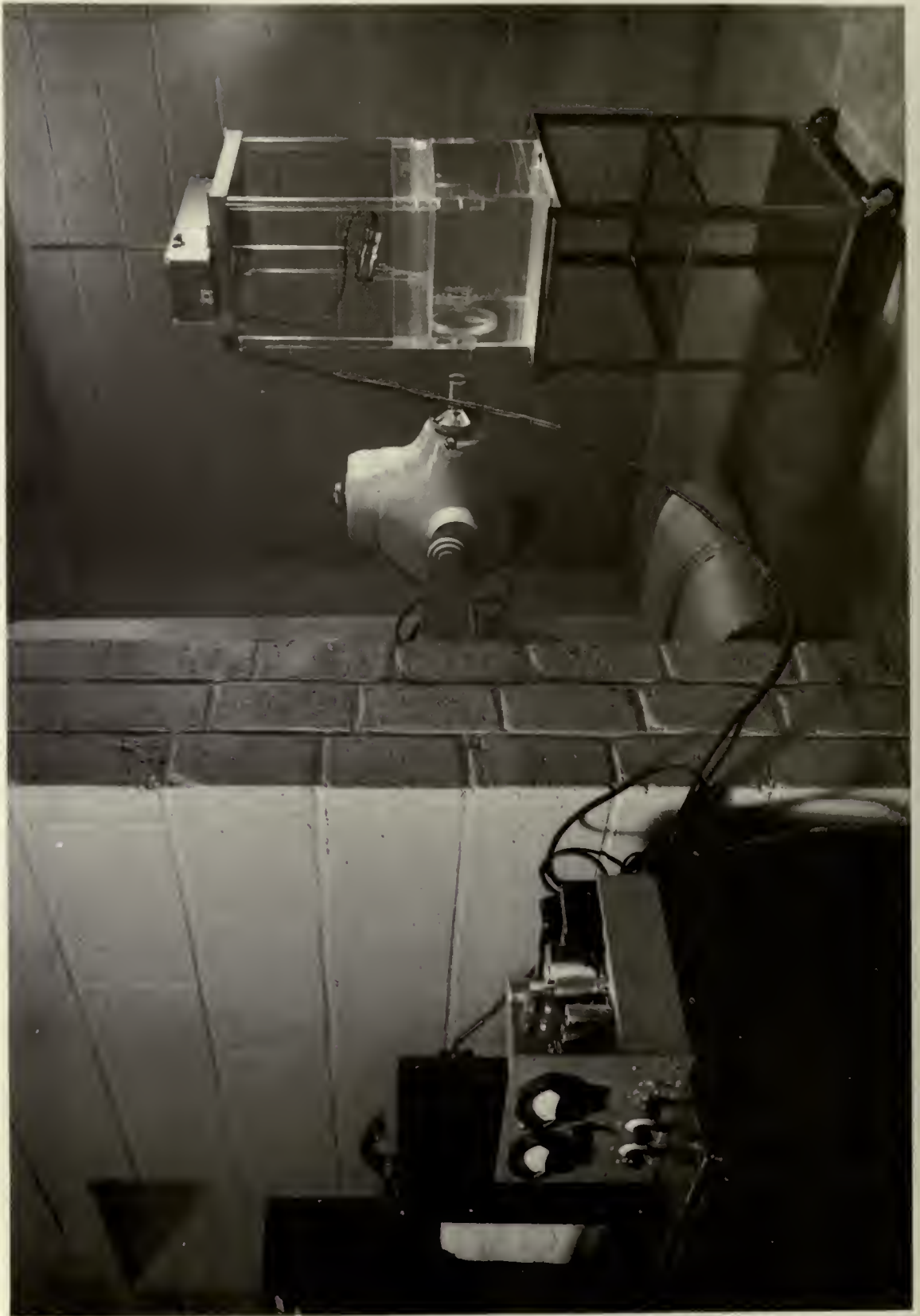
Fig. 2 -- Automatic isodose plotter and amplifier with the teletherapy unit.
