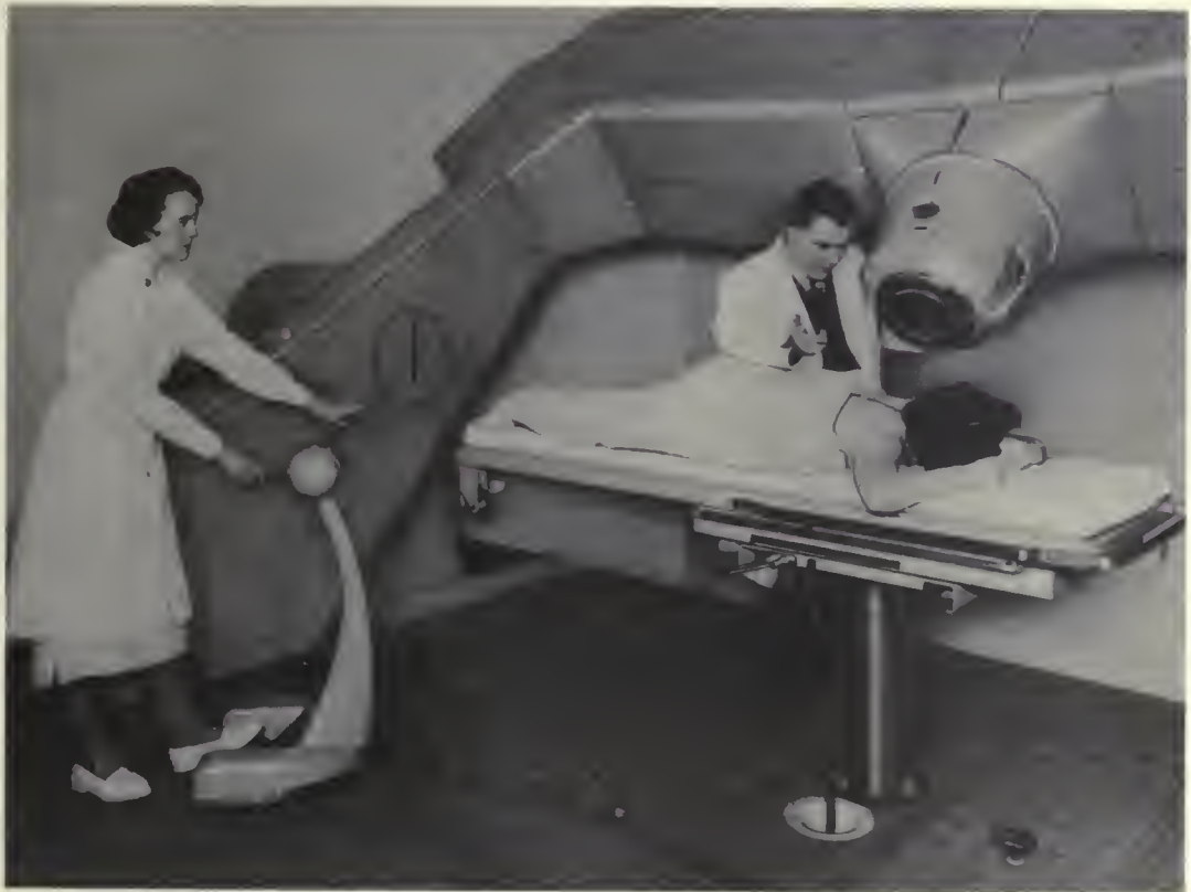
Fig. 5—The 4 million volt linear accelerator mounted on two main bearings, with its single-pillar couch. The movements are designed to facilitate the setting up of fixed fields (with or without an emergent ray pointer) and to allow rotation of the machine about the tumor.
