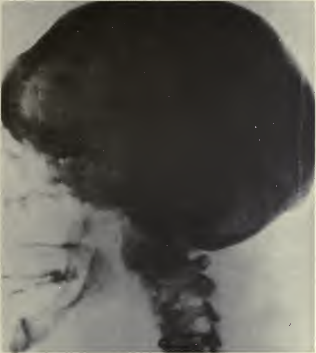
Fig. 20—Contact print produced by exposing phosphor to a light source with intervening X-ray film and subsequently contact printing while the phosphor decayed.
