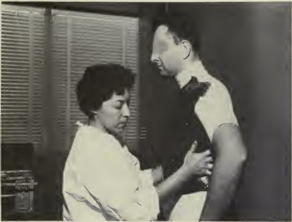
Fig. 1—Method used for molding thermoplastic material about the patient, the first step in preparing a patient phantom to be used for dosage studies.
