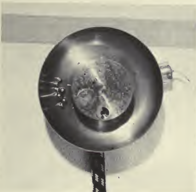
Fig. 8—A view of the vacuum threader, showing the way a \text{Co}^{60} disk is positioned before threading. Note the spherical sources in the catch tray.
