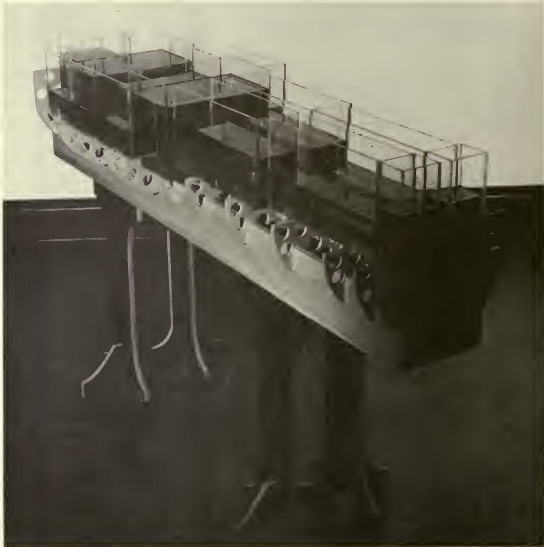
Fig. 1—Compartmentalized standard-man phantom.
