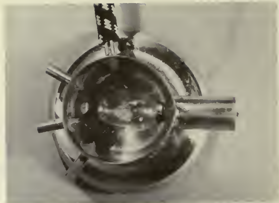
Fig. 1—Vacuum threading device as it appears from the underside. The light source illuminates the threading holes for alignment of the sources before threading. Note the glass elbows in each vacuum line, which allow light transmission.
