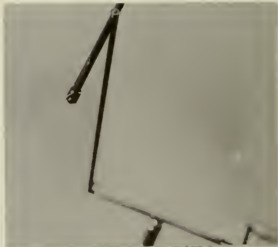
Fig. 4—Vacuum pickup device showing how the thread and the spherical sources are handled.
