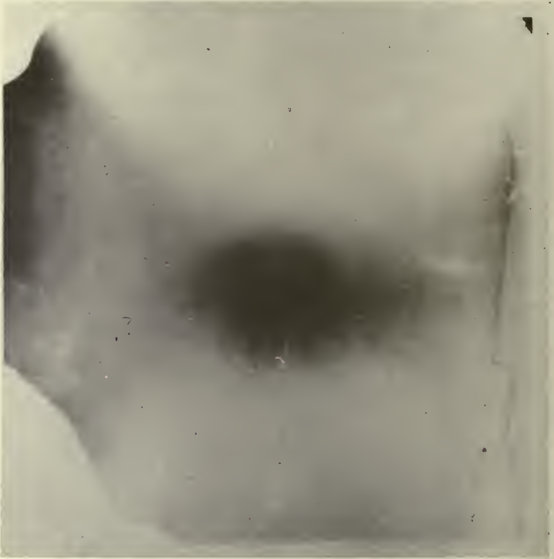
Fig. 19—Contact print on a slow-decay phosphor screen; 270-deg \text{Co}^{60} rotation; Kodak type K film.
