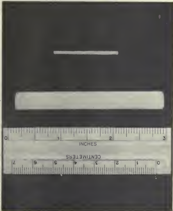
Fig. 4—Cobalt source 7.5 mm by 3 cm is shown with an ordinary cigarette and a ruler.
