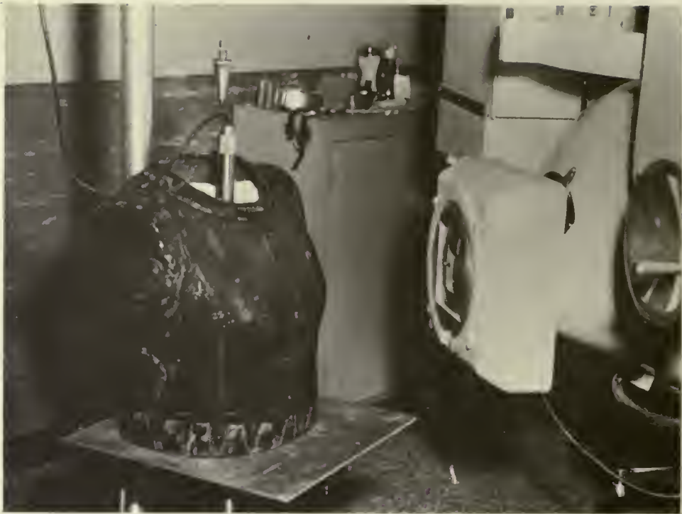
Fig. 5—The Victoreen Radocon is positioned in the chest phantom at the point where the dosage is desired. The phantom is then rotated through the selected arc.
