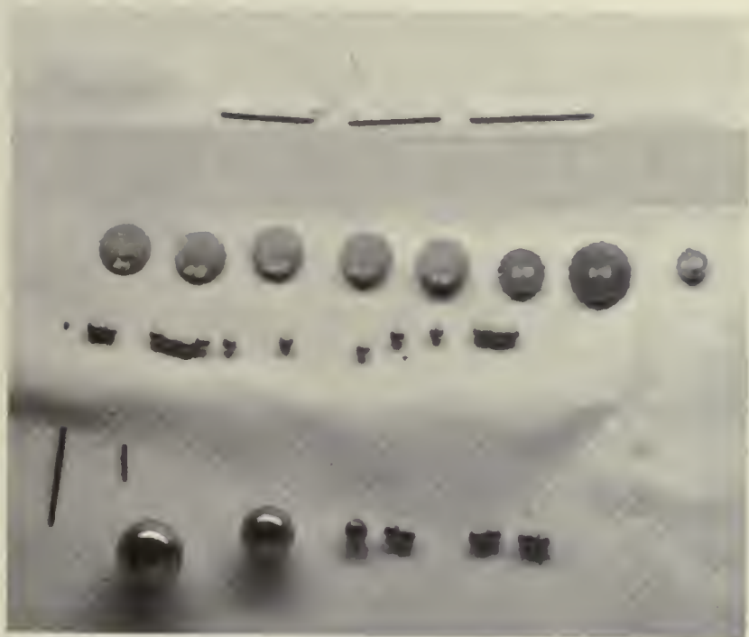
Fig. 7—A view of a variety of brachytherapy \text{Co}^{60} sources through the 9 in. of zinc bromide solution and 1 in. of plate glass.
