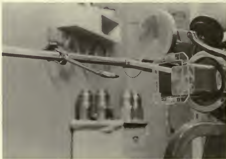
Fig. 4—Back pointer on Keleket-Barnes hectocurie teletherapy unit. A front pointer fits on the device illustrated. This pointer helps to reproduce beam direction after the tumor has been localized by fluoroscopy and by films made with the cobalt machine.
