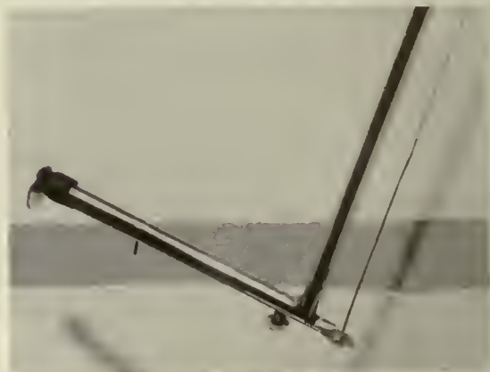
Fig. 5—Vacuum pickup device shown holding a \text{Co}^{60} -alloy disk source.
