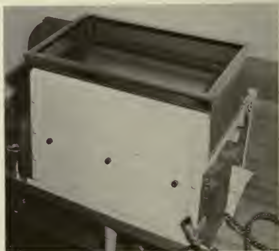
Fig. 6—Zinc bromide viewing tank and associated shielding. Note vacuum control lever in lower right-hand corner.
