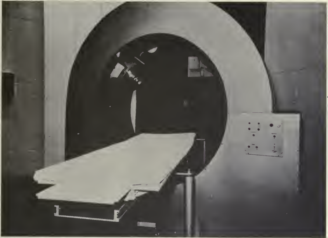
Fig. 3—Completed unit. Panel for set-up operation is at right.
