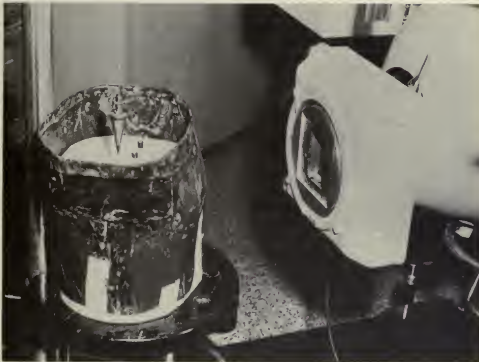
Fig. 3—Cobalt unit and a patient phantom simulating an actual patient arrangement. Note the Phantowax lung cross section and Landsverk ionization chambers.
