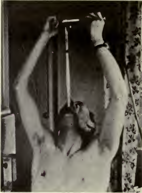
Fig. 4—Continuously reading dose-rate scintillation counter recording dose rate in esophagus during rotation therapy (professional sword swallower).
