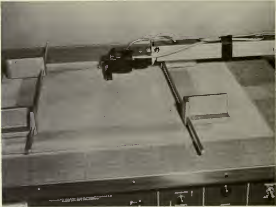
Fig. 21—Automatic isodose plotting device used for scanning X-ray film.
