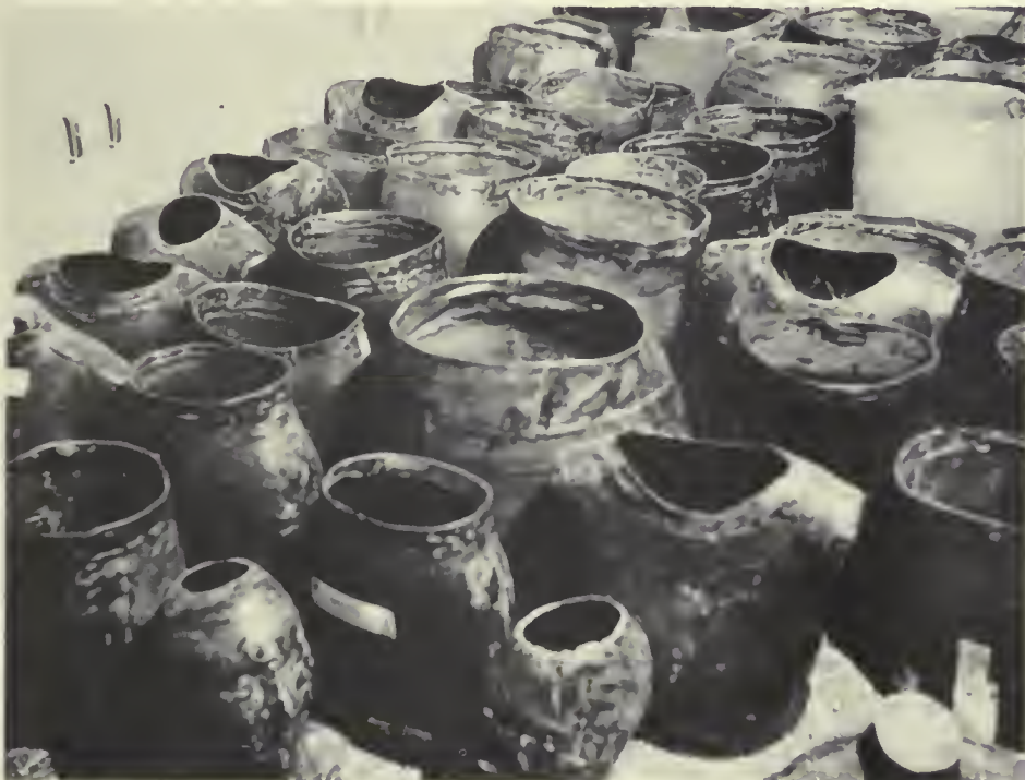
Fig. 2—A variety of patient phantoms made by the technique illustrated in Fig. 1. Phantoms are re-used when dimensions are suitable.
