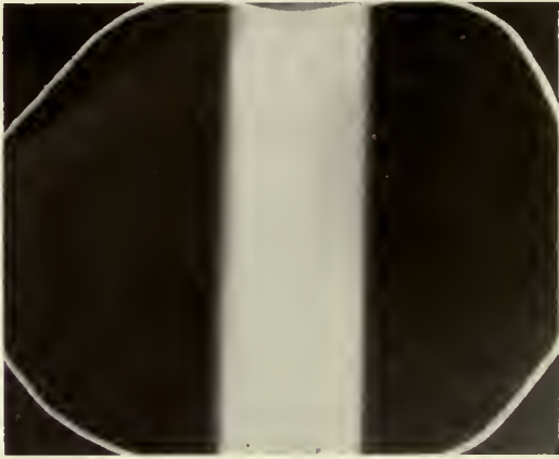
Fig. 1—Radiographic demonstration of a poor type of dose distribution, using supervoltage X rays from a resonant-transformer generator.
