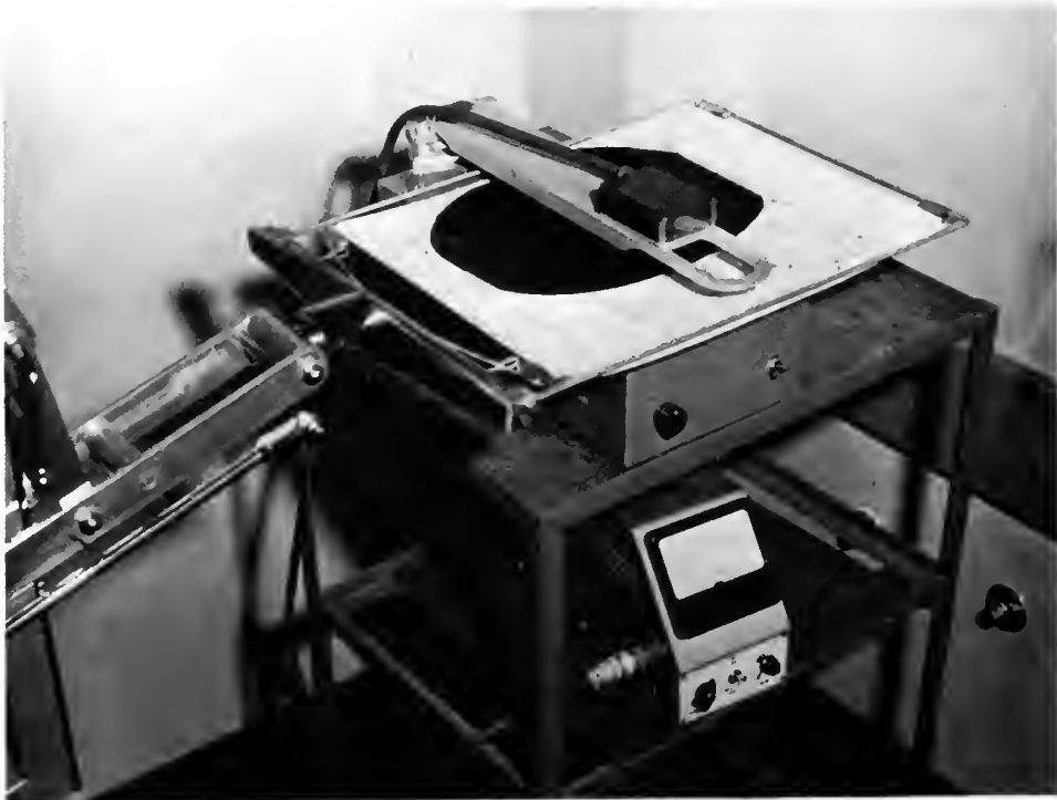
Fig. 22—Scanning arm and densitometer portion of automating film-scanning isodose plotter.
