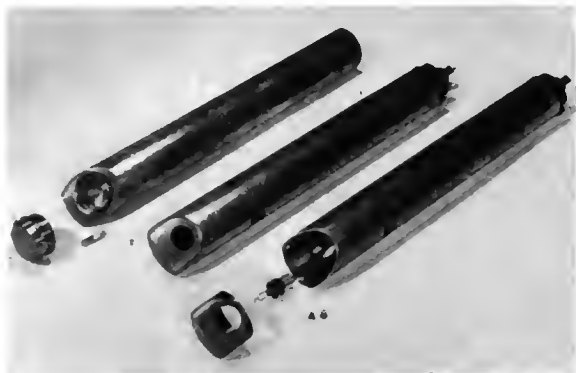
Fig. 6—Cobaltron II source and light pencils.
