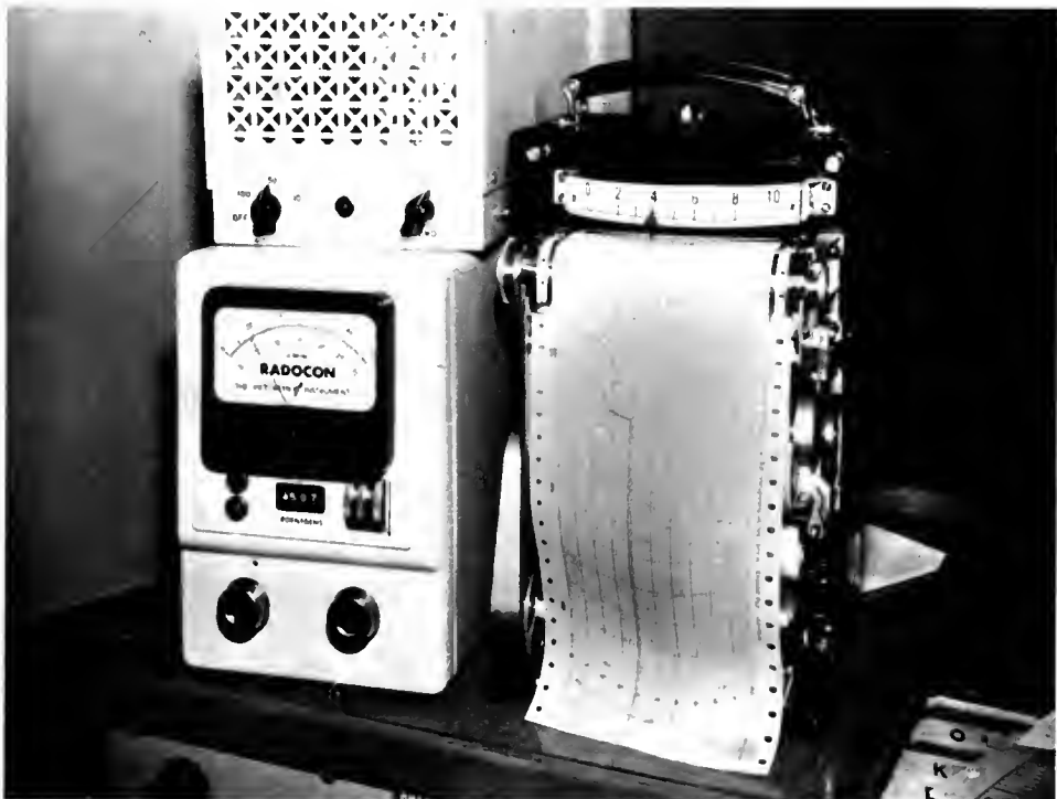
Fig. 6—The Victoreen meter and recorder used for measuring transmission doses and variations of tumor dose as a function of angular position.
