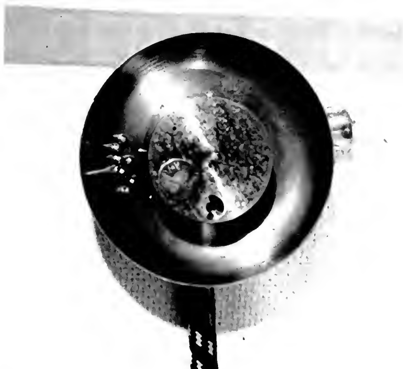
Fig. 8—A view of the vacuum threader, showing the way a \text{Co}^{60} disk is positioned before threading. Note the spherical sources in the catch tray.
