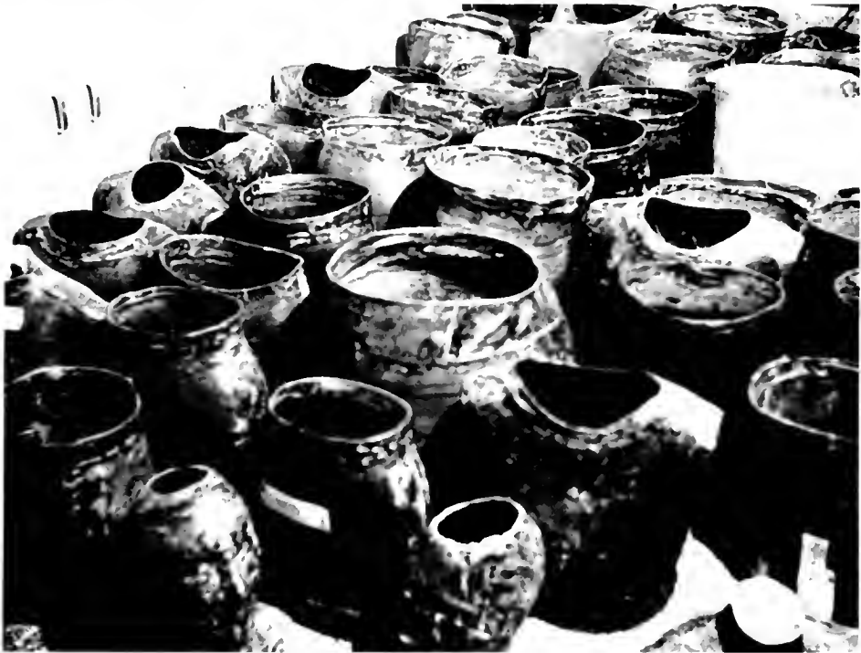
Fig. 2—A variety of patient phantoms made by the technique illustrated in Fig. 1. Phantoms are re-used when dimensions are suitable.
