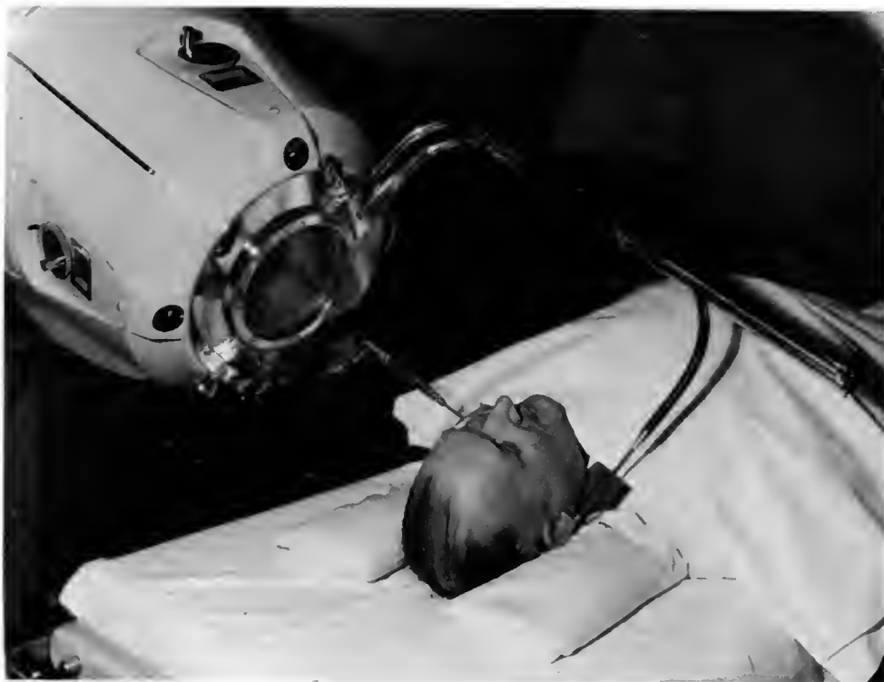
Fig. 6—The 4 million volt linear accelerator with entry and emergent ray pointers. The entry pointer is normally substituted by a 4-beam optical range finder.
