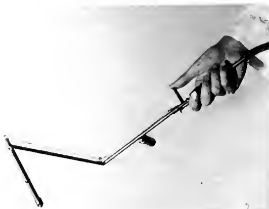
Fig. 3—Vacuum pickup device with thumb-operated clamp for holding the thread during threading. Projection is a counterbalance.
