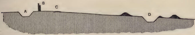
FIG. 20.—Diagrammatic Section of Wall of Hadrian. A, Ditch ; B, Wall ; C, Road ; D, Vallum
