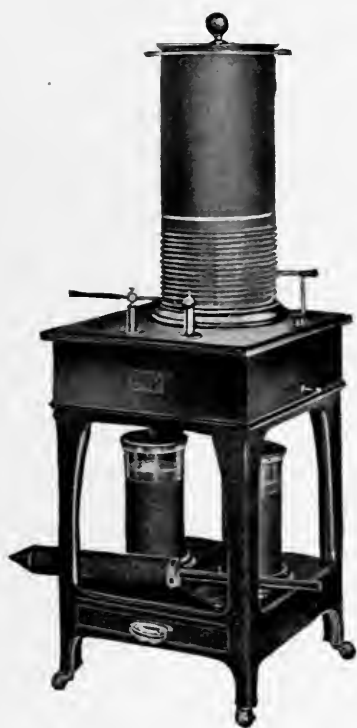
FIG. 61.—Diagram of the Odinn resonator. The Tesla coil is omitted. The current from the induction coil is connected with the inner tin-foil of the Leyden jars. The outer coat of one Leyden jar is in connection with the resonator, and is also grounded. The outer coat of the other Leyden jar is connected to the handle, H , which, by a sliding movement either in the vertical or the horizontal direction, decreases or increases the amount of winding of the resonator. M is the spark-gap for regulating the amount of current.
