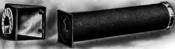
FIG. 217.—The improved benoist radiochromometer.
