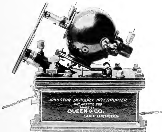
FIG. 73.—Johnston's mercury interrupter.
