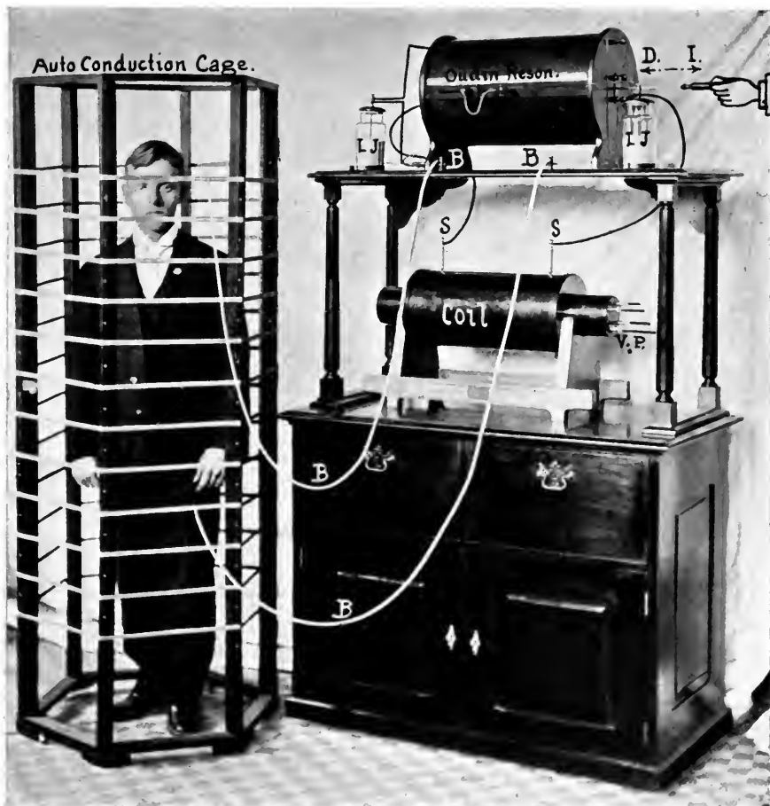
FIG. 66.—Treatment by auto-conduction. S S , secondary terminals of induction coil; B B , cords to the auto-conduction cage from the Oudin resonator; L J , Leyden jar; D. ↔ I. , spark-gap; when sliding in the direction " D ," the current suffers a loss in intensity, and vice versa.
