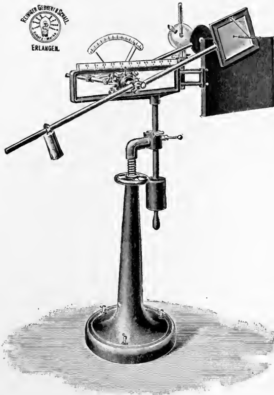
FIG. 181.—Levy-Dorn's orthodiagraph for the standing position.
