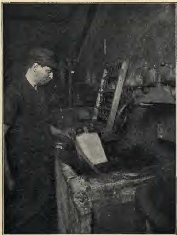
The Electrotyper, taking the Copper Shell from the Mold.
