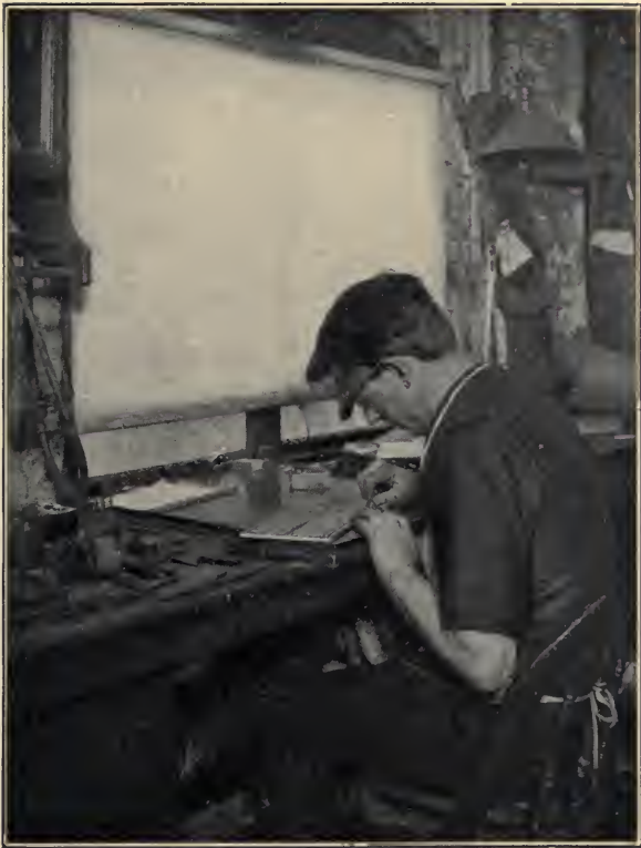
The "Finisher," who gives the final touches to the Electrotype Plates.
