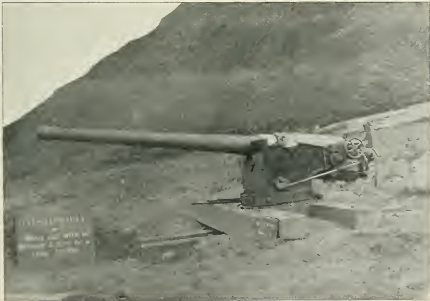
4.7 IN. Q.-F. GUN, FROM THE "TERRIBLE," ON SCOTT'S PLATFORM MOUNTING, AT LADYSMITH.
