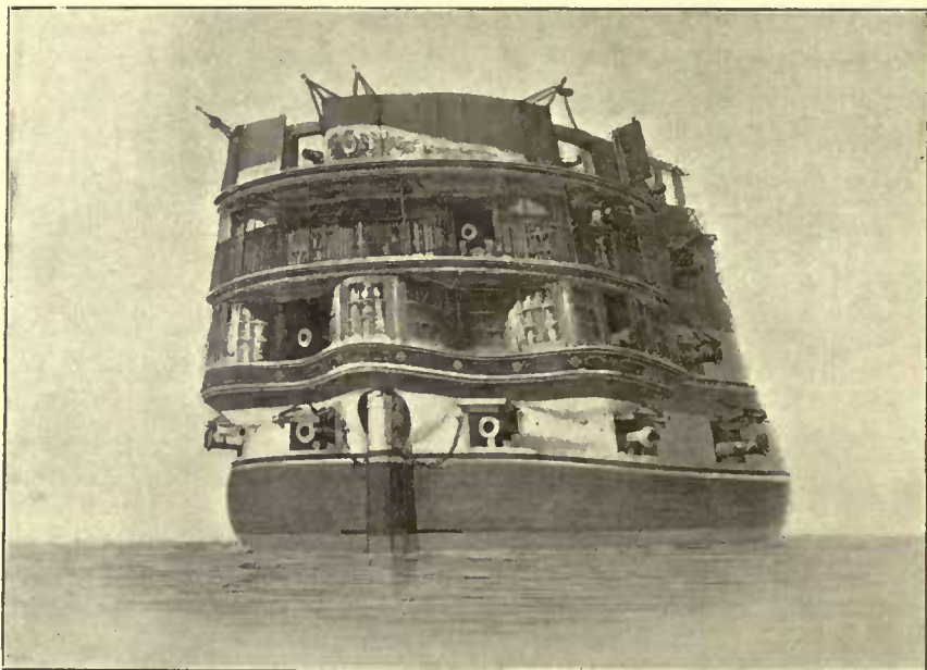
CIRCULAR STERN OF H.M.S. 'ASIA,' 84, BUILT AT BOMBAY, 1824. FLAGSHIP AT NAVARINO.
