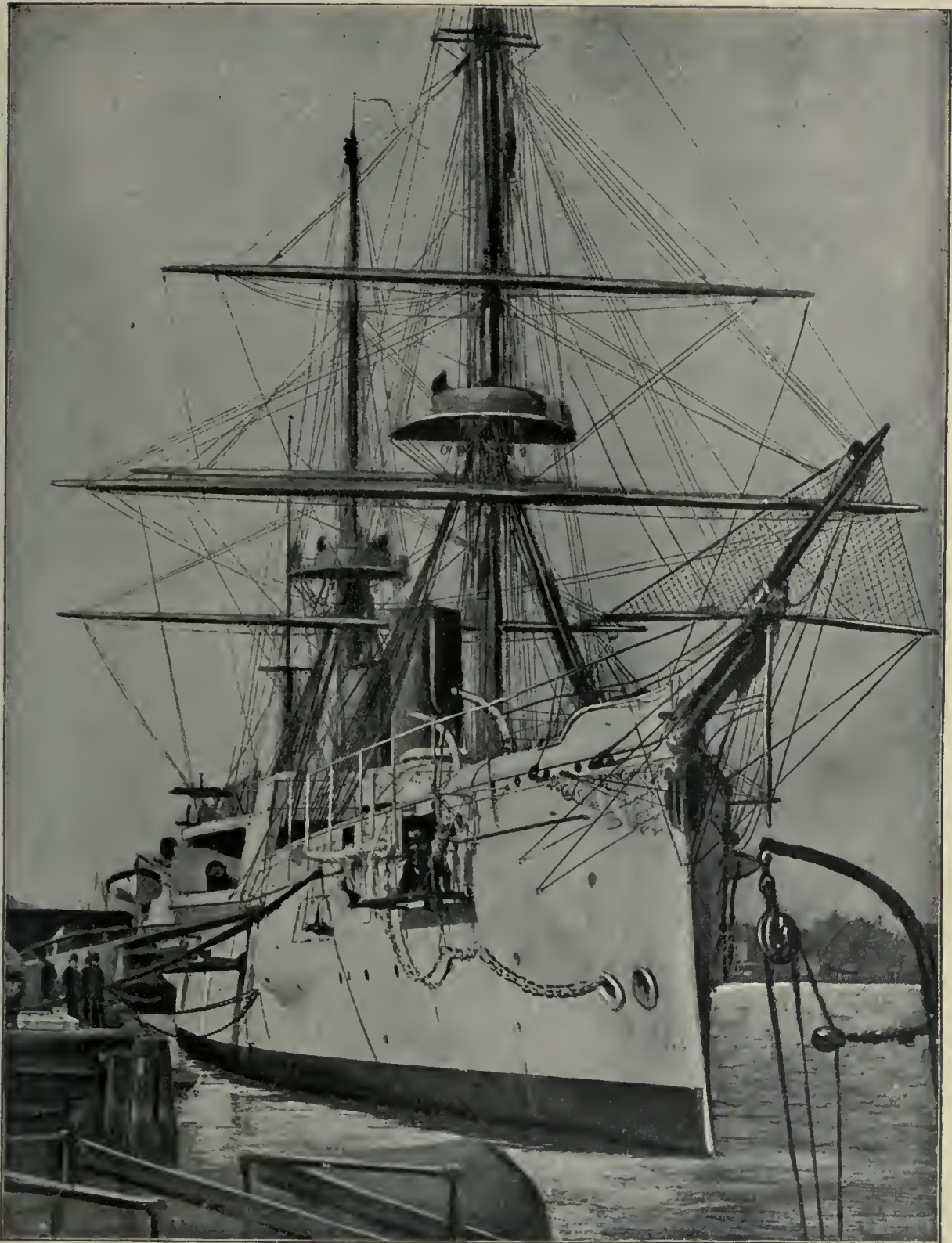
NEW YORK NAVY YARD: THE "CHICAGO." —This beautiful vessel is of the type partially protected cruiser; her hull is of steel, she is propelled by twin screws, is bark-rigged, carries fourteen guns in her main battery and twenty-seven in all, and has a displacement of 4500 tons. She is painted white and presents a very pleasing appearance. The "Chicago" was Rear-Admiral Walker's flagship in the great international pageant at Hampton Roads, in April, 1893, that gallant seaman being in command of the second squadron. Her construction was authorized by Congress in 1883, with that of the cruisers "Boston" and "Atlanta" and the despatch-boat "Dolphin." This last-named was the first United States vessel, either naval or commercial, built entirely of steel of domestic manufacture.
