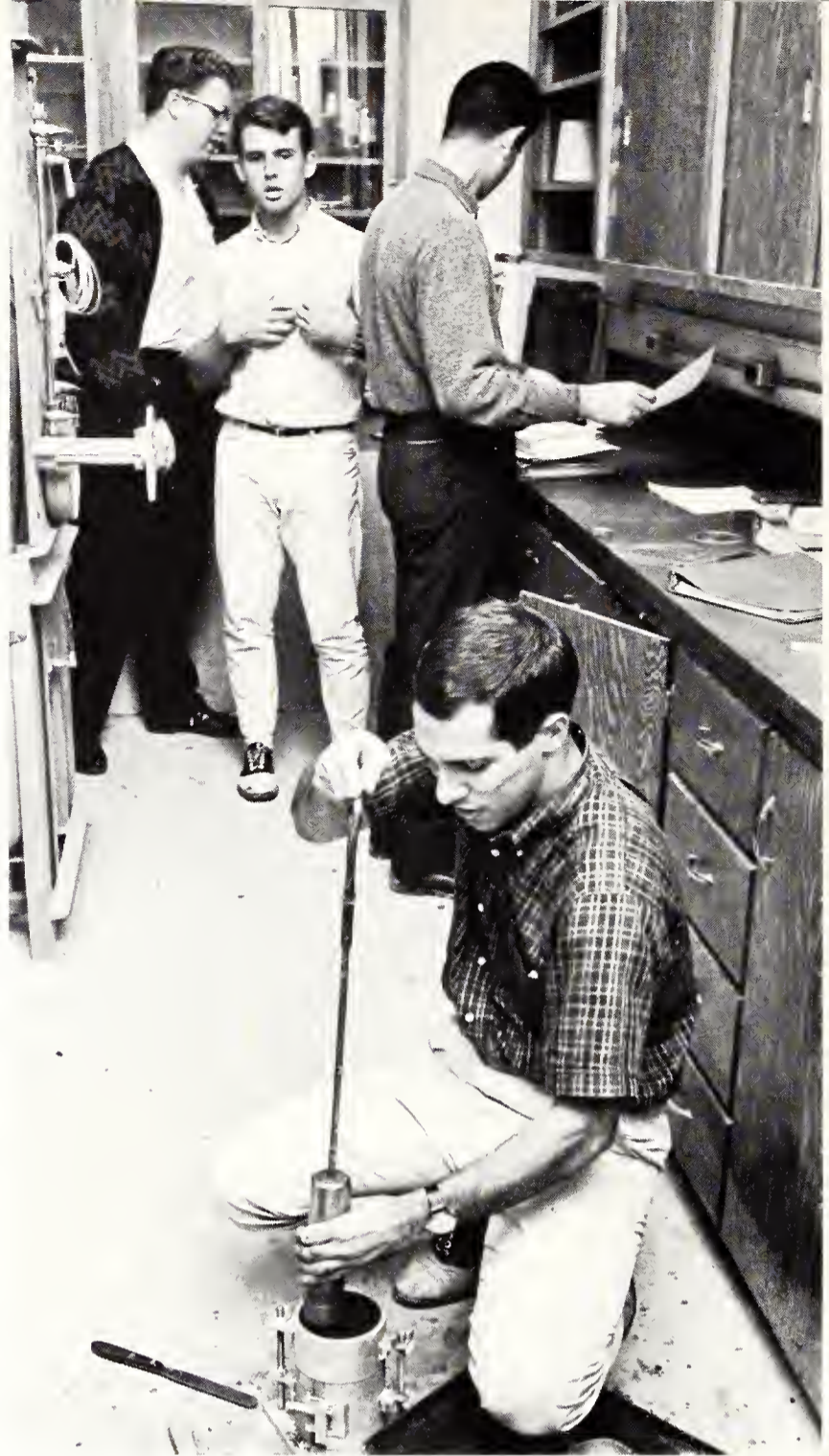
Through a soil compaction test during a soils laboratory period, students attempt to find optimum moisture content.
