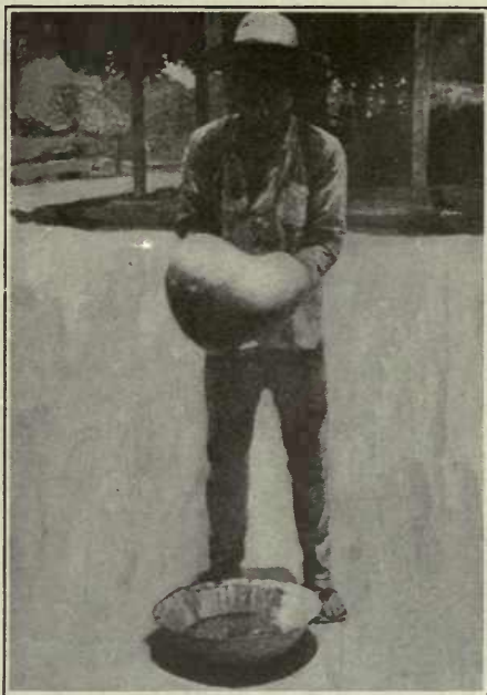
FIG. 16—COAGULATING WITH VINE JUICE
