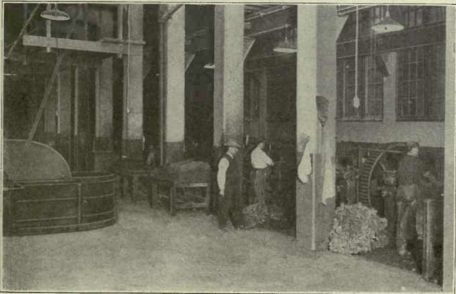
FIG. 35—WASHING AND SHEETING RUBBER
