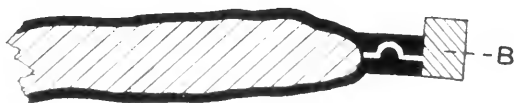
FIG. 4. Detail section through beak region showing second half of the mold and the plasteline dam in place. B, plasteline dam.
