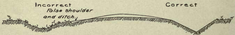
Fig. 3. Second ditch and false shoulder as often left in regrading. Correct form shown at the right.
