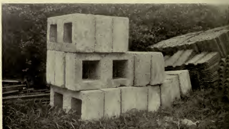
FIG. 29.—Concrete blocks used in construction of the houses shown in Fig. 27 and Fig. 28.
