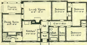
First Floor Plan
