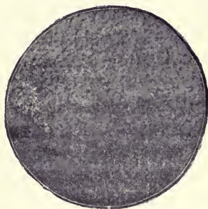
FIG. 26.—Deposit from zinc sulphate solution (acid), magnified five diameters.
