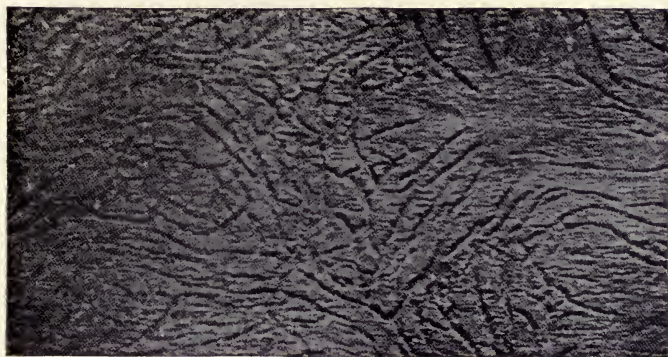
FIG. 67.—Hardened steel (polished). Magnified 2\frac{1}{2} diameters
