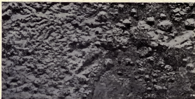
FIG. 63.—Burned steel not hardened (with scale). Magnified 2\frac{1}{8} diameters.
