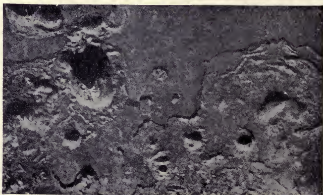
FIG. 65.—Annealed steel (with scale). Magnified 2\frac{1}{8} diameters.
