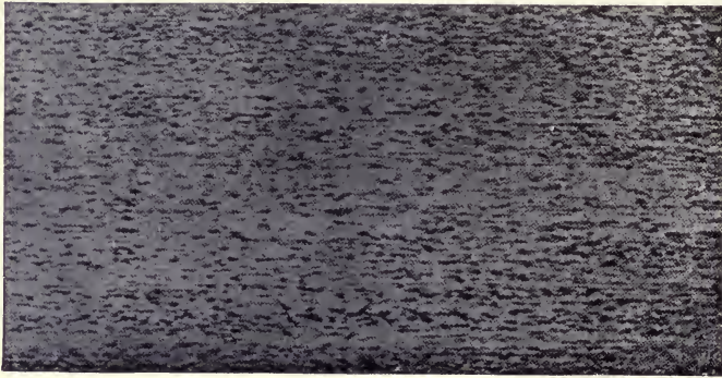
FIG. 58.—Mild steel (ammonium-chloride solution). Magnified 2\frac{1}{2} diameters.
