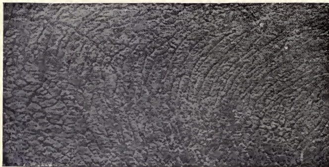
FIG. 69.—Steel burned and hardened (polished). Magnified 2\frac{1}{3} diameters.
