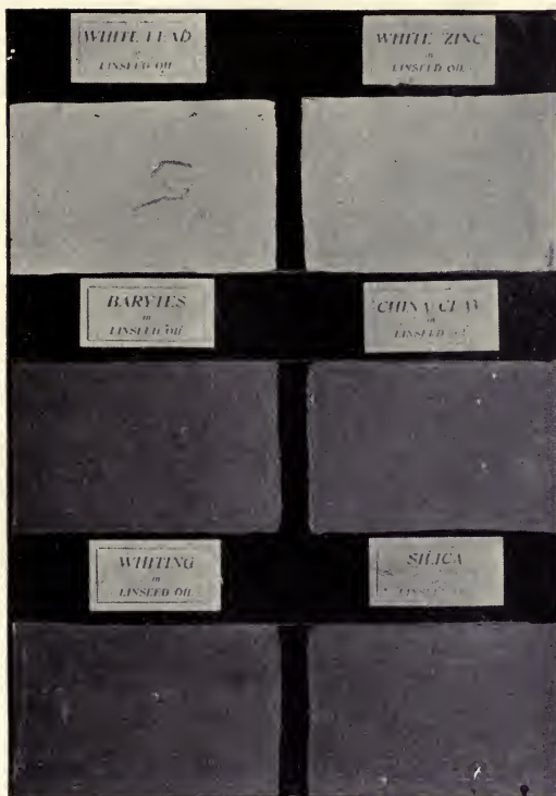
FIG. 29.—Covering power of inert pigments.
