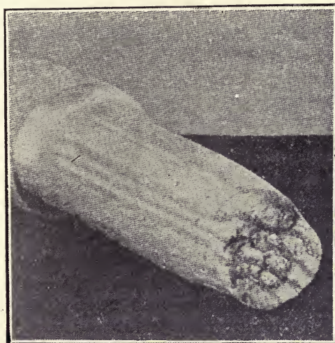
FIG. 51.—Effect of strain on the corrosion of iron.
