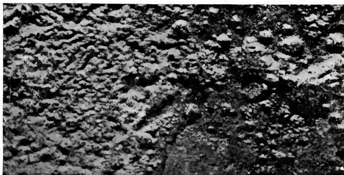
FIG. 63.—Burned steel not hardened (with scale). Magnified 2\frac{1}{2} diameters.
