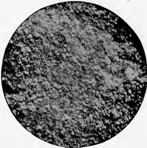
FIG. 4.—Rust produced on a clean rolled-iron plate exposed to atmospheric influences for 20 days. (Andes.)
