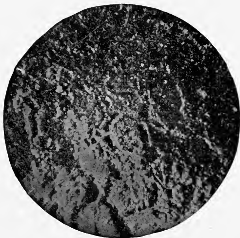
FIG. 8.—Dried film of red lead encrusted with rust \times 100 . Taken from a painted structure which showed no rust on surface. (M. Toch.)
