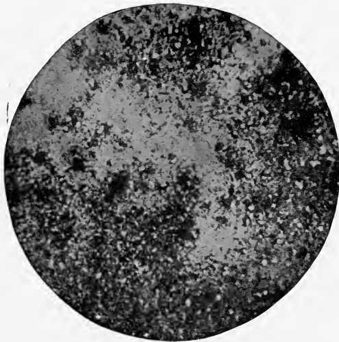
FIG. 10.—Photomicrograph \times 100 of red lead and oil taken from a paint-pot and dried on a slide. The film is filled with air-bubbles and the coat is transparent in spots, although to the eye it looks solid. (M. Toch.)
