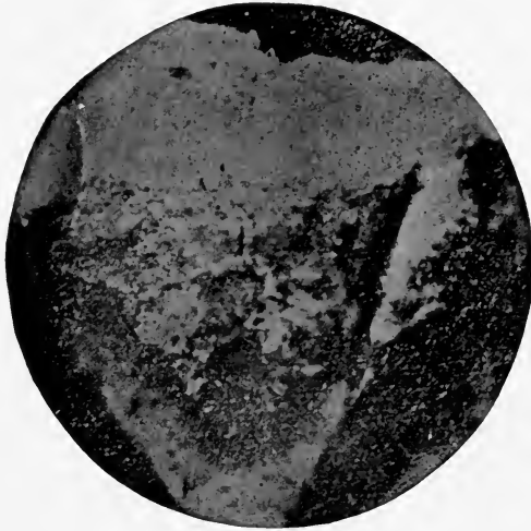
FIG. 11.—Photomicrograph \times 100 of a film of dried paint taken from an iron pillar showing rust blisters. The dark spot is red lead and a fissure runs through the centre. The zinc oxide and white lead are white and are intact. (M. Toch.)
