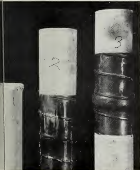
Fig. 4—Joints 1 and 2 (shown also in scale sections on Fig. 1 and a section of similar asbestos cement pipe for comparison. No tension test was made, but compression tests destroyed joint 1 (center) at 21,000 lb. and joint 2 (right) at 18,000 lb. The pipe (left) failed in compression at 2200 lb., showing that the joints weakened the pipe. Fig. 5—(Right) Testing machine in the Talbot laboratory on which all the tests were made. The joint being tested is shown in Fig. 1 as No. 5, the 6-in. pipe coupling
