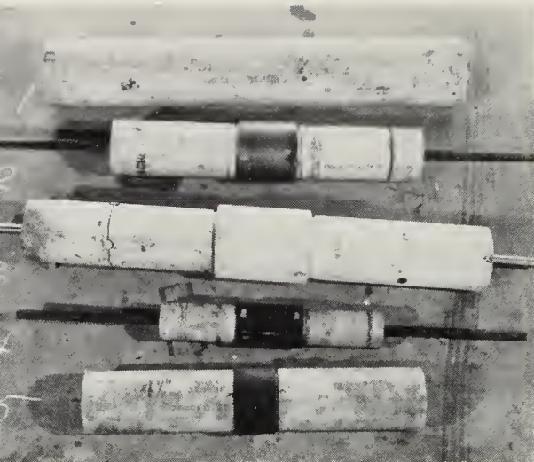
Fig. 2—(Left) A section of asbestos cement pipe at 1, joint 4 at 2, joint 6 at 3, joint 3 at 4, and joint 5 at 5
