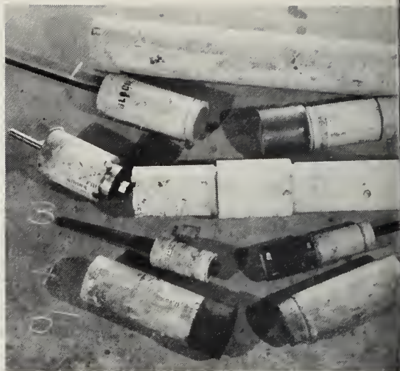
Fig. 3—(Right) The joints after being tested to failure. Points of failure are indicated for each joint in Fig.
