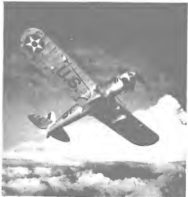
The PT-20A, manufactured for the Army, was the first model of the Ryan training plane to be equipped with a radial engine.
