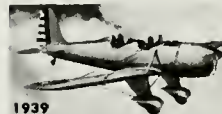
1939 RYAN STM, first low-wing primary trainer types (PT-16 and PT-20) used by Army.
