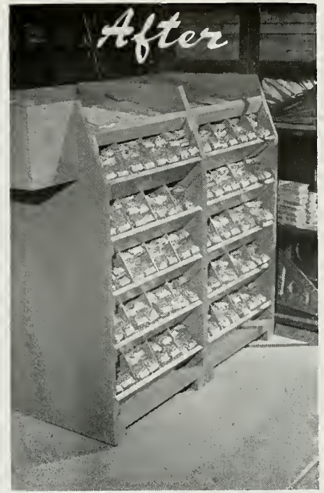
Everything neatly sorted and labeled, with no way for rivets to get spilled, mixed, or used on the wrong job. Riveters enthuse about the new plan.
