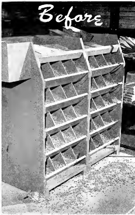
The standard type of rivet rack, open for anyone to reach in and take a handful. It's obvious how many chances for confusion and waste there were!
