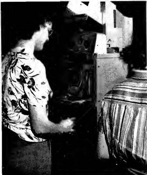
A special weighing machine fills the bags. It trips automatically when the correct weight is poured into a bag.
