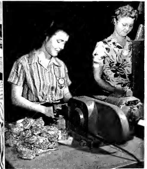
The cellophane bag is sealed in another machine which closes the end by means of heat and pressure.
