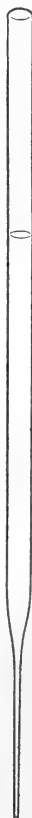
FIG. 30.—Capillary pipette. A piece of glass tubing drawn to capillary size at one end. Reduced to three-fourths of the size used. (Original.)
