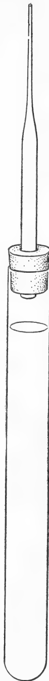
Fig. 31.—Tube in which a suspension of sacbrood larvæ is placed for heating. It consists of a test tube one-half inch in diameter supplied with a perforated stopper through which passes a short piece of glass tubing drawn at one end to capillary size. (Original.)
