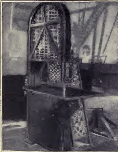
THE OLIVER IRON MINING COMPANY'S BAND-SAWS PROTECTED BY WIRE-MESH GUARDS
