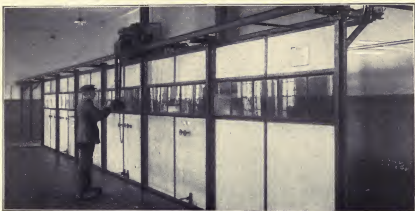
AUTOMATIC ACID-DIPPING PROCESS IN USE AT THE ALLGEMEINE ELEKTRICITAETS GESELLSCHAFT. NO INHALATION OF FUMES OR CONTACT WITH THE ACID
