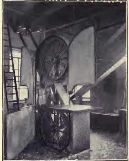
METAL SHIELDS FOR BAND-SAWS IN SHOPS OF ILLINOIS STEEL COMPANY
