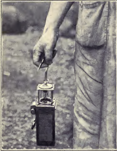
THE EDISON PORTABLE SAFETY LAMP FOR MINERS
