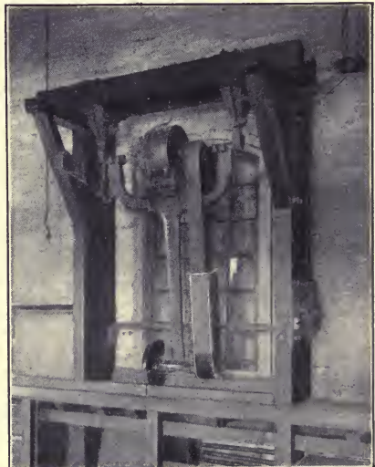
A PENDULUM SAW WITH METAL HOOD AND COUNTERWEIGHT IN CARPENTER SHOP OF THE NATIONAL TUBE COMPANY
