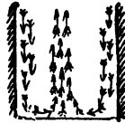
Fig. 110.—Down and Up Currents in Large Shafts.
