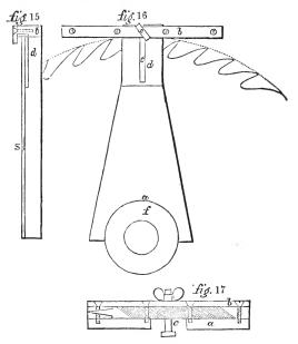
same tool in position on the saw. To use this tool, place the open end astride the collar, and bring the file down to the shortest tooth, or to the edge of the one which is at the least distance from the centre of the saw, and screw it fast; then pressing it down on the collar, and against the side of the saw, move the file forward until the edges of the teeth are at the same distance from the saw centre.
