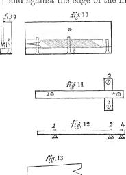
position, seen in Fig. 10. Fig. 9, is an end view of the file gauge position in the saw ready for use. To use this tool, apply it to the side of the saw with the file on that part of the teeth set out, when a few strokes
