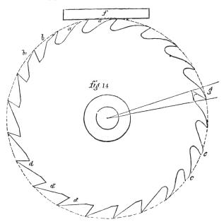
Sec. 2. Gauge.—The gauge depends upon their quality of steel, their number of teeth, and their diameter. The larger their diameter, the thicker they must be in order to work with firmness. Good temper and finer teeth may reduce the gauge somewhat.
