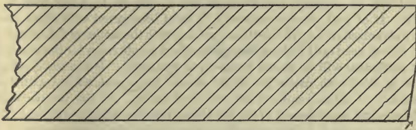
FIG. 8.—Plank showing beveled edge for calking.
