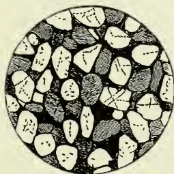
FIG. 21.—Ordinary Unaltered Red Sandstone (Cambrian), Keeshorn, Ross-shire (magnified), showing the irregularly-shaped grains of quartz, felspar, etc.
