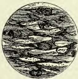
FIG. 22.—Sheared Red Sandstone forming now a Micaceous Schist, Keeshorn, Ross-shire. The pebbles are crushed and elongated, and the felspar materials have been partly converted into mica.
