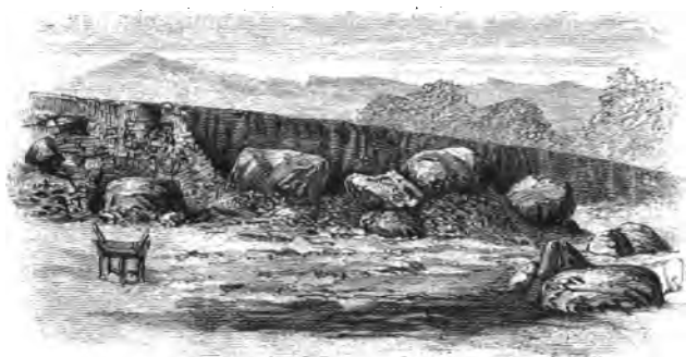
FIG. 83.—Section of Boulder-Clay, Craiglockhart Hill, Edinburgh. Exposed when the foundations of the Hydropathic Establishment were being dug out.
