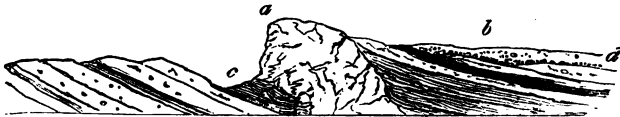
FIG. 82.—Section of the form of hill in the Lowlands of Scotland known as 'Crag and Tail.' a , 'Crag' of basalt or other eruptive rock. b , 'Tail' of softer rocks which have been worn away from around the hard igneous mass. c , Hollow often found in front of the crag. d , Covering of drift.
