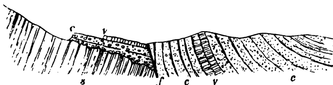
FIG. 30.—Section across the boundary fault of the Highlands at Glen Turril, Perthshire. s , Crystalline schists of the Highlands. c , Conglomerate and sandstone (Old Red Sandstone), with vv , associated volcanic rocks. f , Fault.
