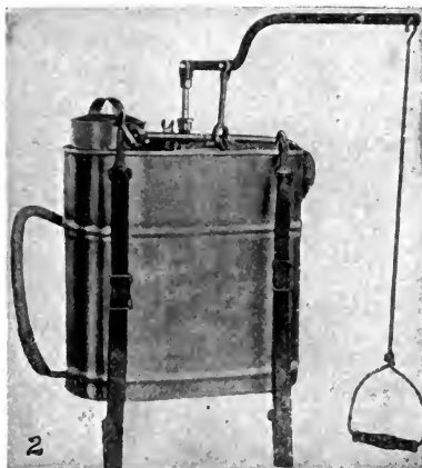
FIG. 147.—Knapsack sprayer, suitable for use in fighting garden pests. (Fights of the Farmer.)
