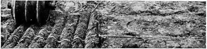
FIG. 68.—The soil packer shown here leaves the surface slightly ridged but loose—an ideal seed bed for the garden. (Dunham Co., Berea, Ohio.)
