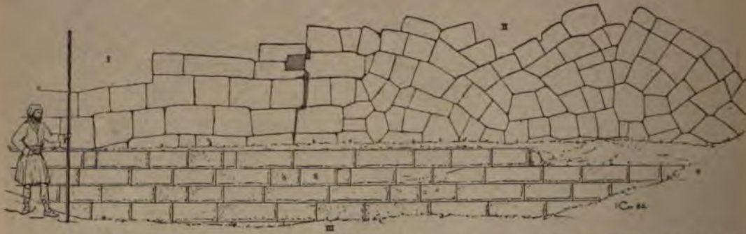
FIG. 2.—Corner of oldest polygonal city wall (I.), with extension in irregular masonry antedating the Persian wars (II.); both reveted, after the age of Lysimachos, with an escarpment of squared blocks (III.).
