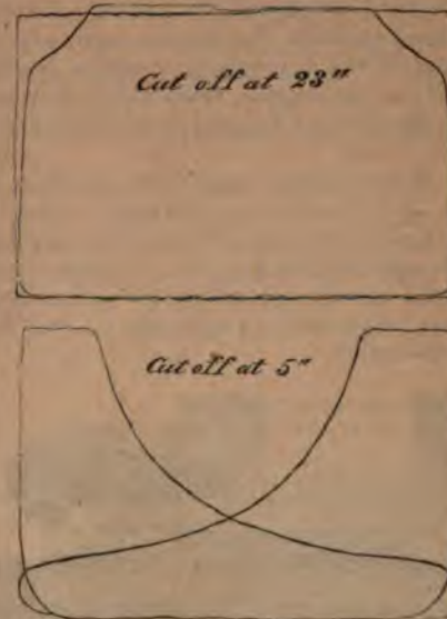
INDICATOR DIAGRAMS OBTAINED ON LOCOMOTIVE BUILT AT THE COOKE LOCOMOTIVE WORKS.
