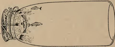
A "Lead in" that makes a Minnow Trap of an Ordinary Glass Jar.
