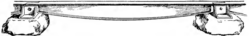
Edge Rail, Patented by Losh and Stephenson, laid on Stockton and Darlington Railroad, A. D. 1816.
