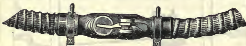
Hose coupling between the cars, through which the air passes in order to operate the brakes on the cars.
