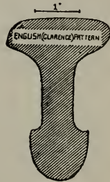
Rolled Rail, Old Portage Railroad of Pennsylvania, A. D. 1833.
