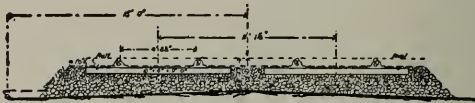
Section of double track, New South Wales. Top ballast broken blue stone 2½-inch gauge; bottom ballast broken stone, 4-inch gauge, hand packed.
